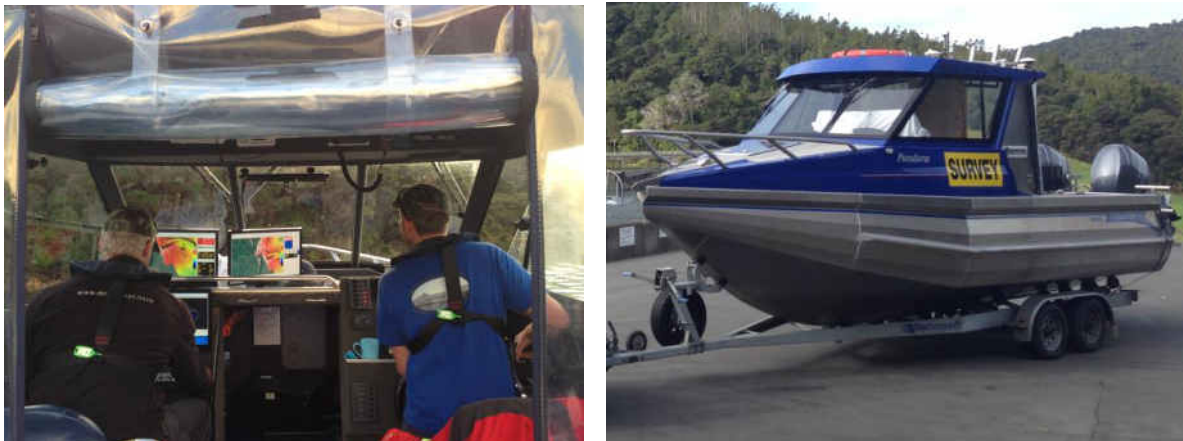
Photograph 2: 7m vessel with survey grade MBES fitted
