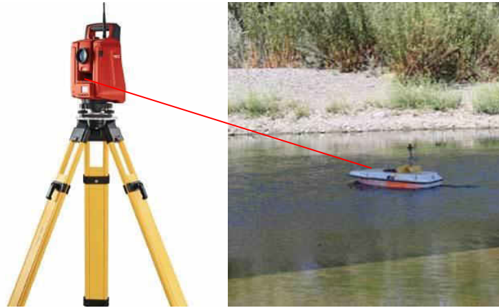
Figure 5: Robotic total station coupled with a USV
