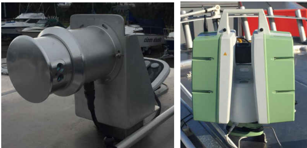
Photograph 3: Mobile laser scanners mounted to a 7m vessel
