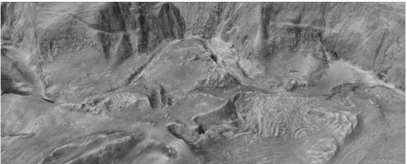
Figure 22: Backscatter imagery draped over bathymetry, Lower Huia Dam
