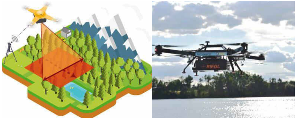
Figure 7: UAV fitted with Lidar
