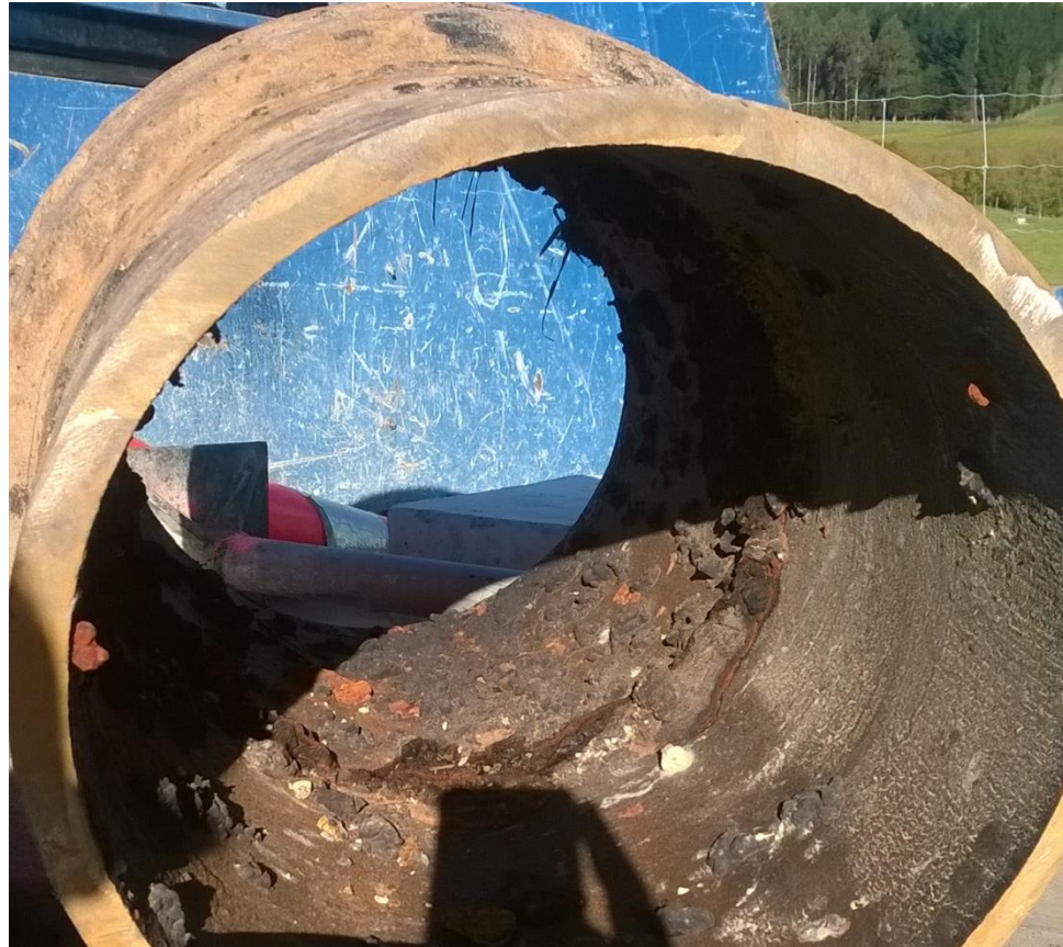
Sample of DN375 Cast Iron Watermain 150 years old.
